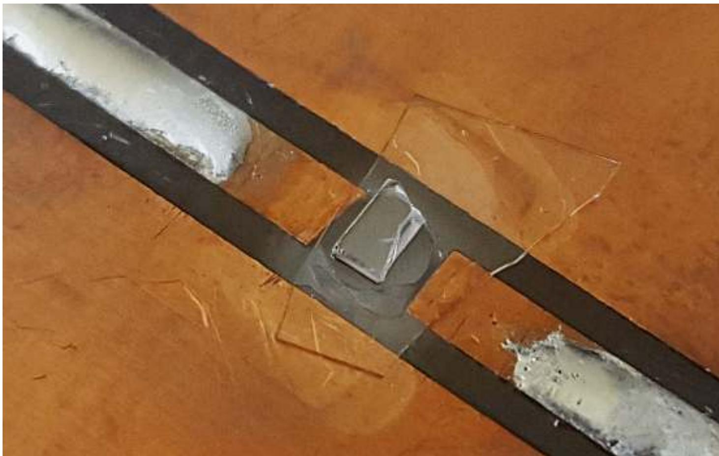
A team led by Fedor Jelezko, director of the Institute for Quantum Optics at Ulm University in Germany, probed the state of a nitrogen “defect” inside a synthetic diamond (shown mounted on the right) by monitoring surrounding carbon atoms. Their findings confirmed predictions of a theory known as quantum Darwinism.
