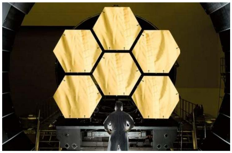
NASA engineer Ernie Wright supervises the instalation of the first six primary mirror segments from the James Webb Space Telescope to begin the final round of cryogenic test at NASA's Marshall Space Flight Center.
