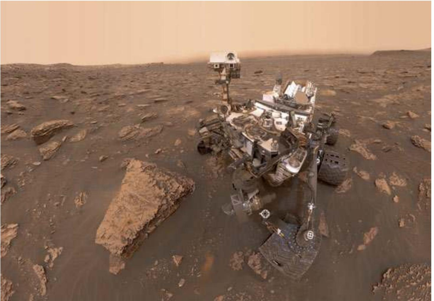
A self-portrait by NASA's Curiosity rover taken on Sol 2082 (June 15, 2018). A Martian dust storm has reduced sunlight and visibility at the rover's location in Gale Crater. A drill hole can be seen in the rock to the left of the rover at a target site called "Duluth"
