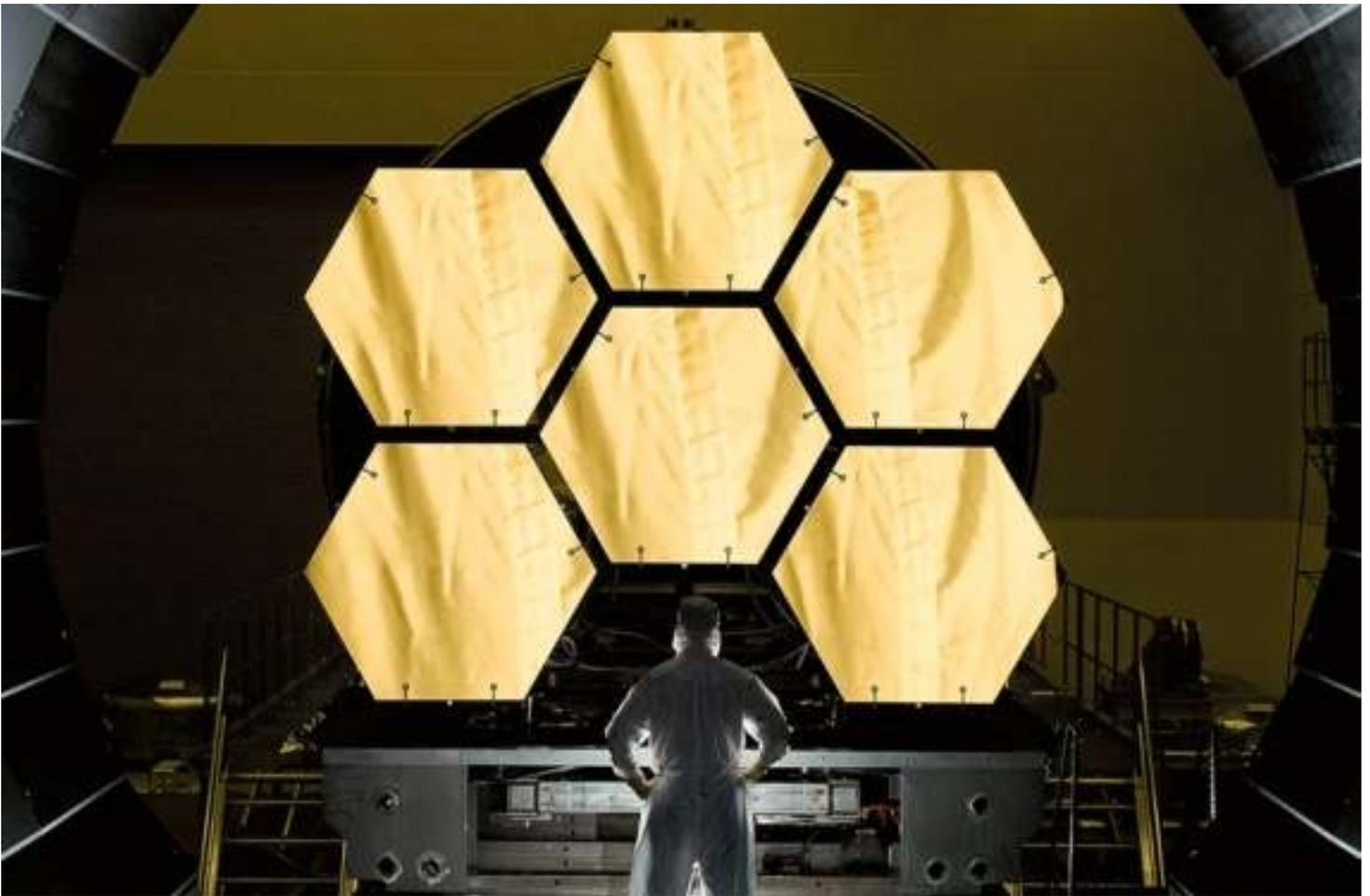
NASA engineer Ernie Wright supervises the installation of the first six primary mirror segments from the James Webb Space Telescope to begin the final round of cryogenic test at NASA's Marshall Space Flight Center.
